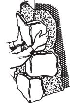
Figure 11 Applying corners— alternating long and short legs in the opposite direction
